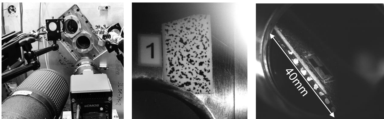
Fig. 2 left: Radial camera setup for simultaneous acquisition of speckle pattern on the hub (center) and near the blade root (right); Center: image of the hub tracking camera; right: simultaneously acquired image of the blade tip with painted dot pattern and reference marker.
