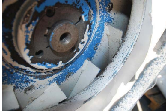
Fig. 9: Erosion damage to the central hub area and no damage to the blade suction side
