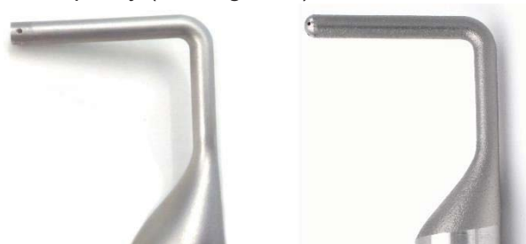
Figure 2: 3D-printed L-shaped probe head: After 3D-printing (left) and after post manufacturing (right)
