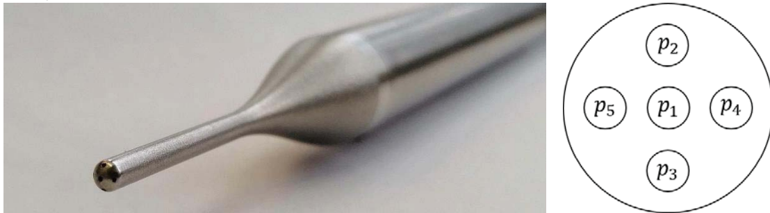
Figure 1: 3D-printed straight unsteady five-hole pressure probe and numeration of holes
