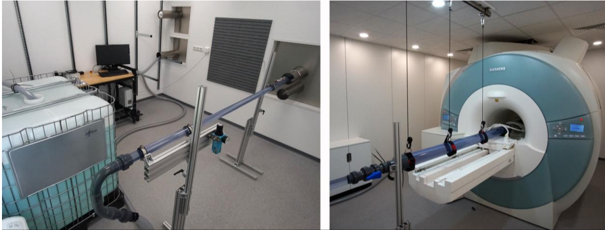
Fig. 4 Pictures of the experiments with the stenosis test case. A straight pipe, shown on both image parts, connects the pump system with the flow model in the MRI system.
