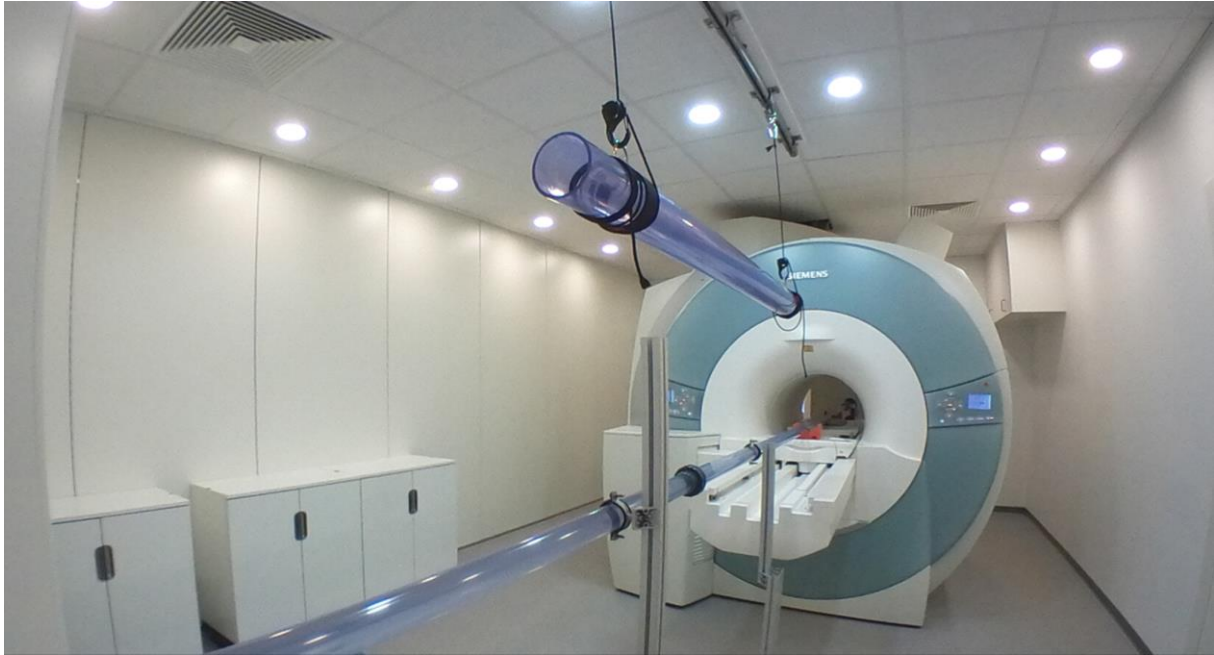
Fig. 1 Picture of the MRI flow lab showing the MRI scanner and a flow circuit installation.
