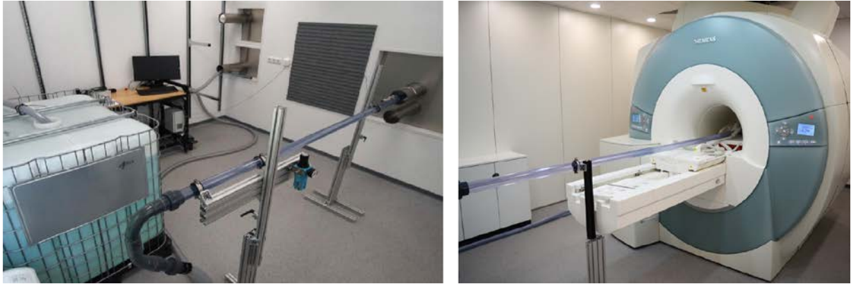
Fig 2: Pictures of the experimental set-up. A straight pipe, shown on both image parts, connects the pump system with the flow model in the MRI system.
