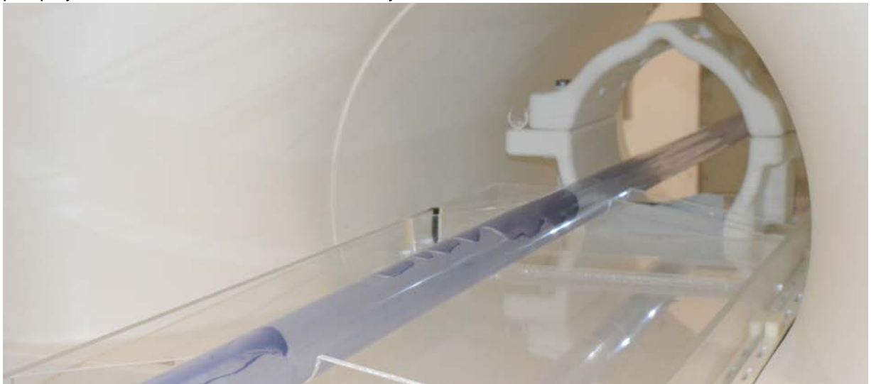
Fig 3: Picture of the two-phase flow experiment with 1-channel head coil for MRI-measurements.
