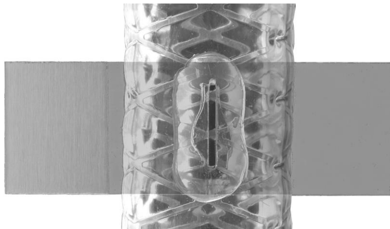
Figure 7: Flat glass plate for positioning the measuring volume and proofing the gas flow
