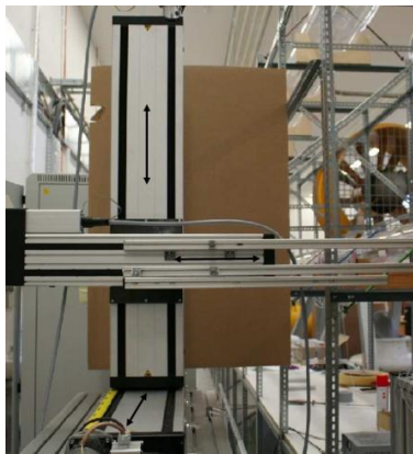
Figure 6: (left) Traverse mechanism able to move in x-, y- and z- directions Figure 7: (right) Placement of probe and probe support in the test section
