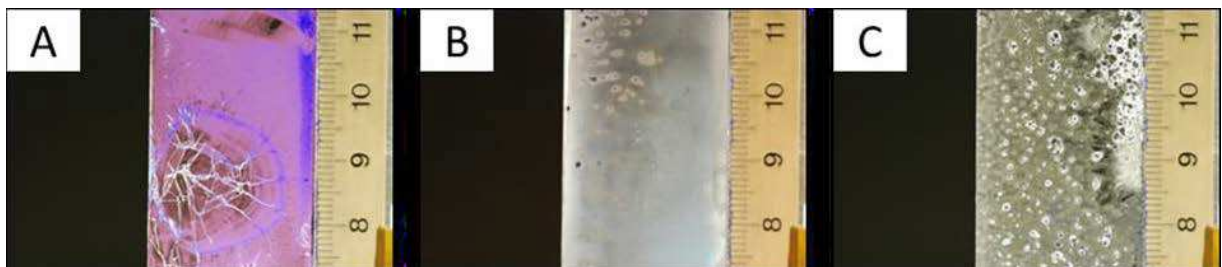
Fig. 3. Results after 10 min. of treatment with Al-Fe electrodes (A-olive oil, B-milk and C-eggs)
